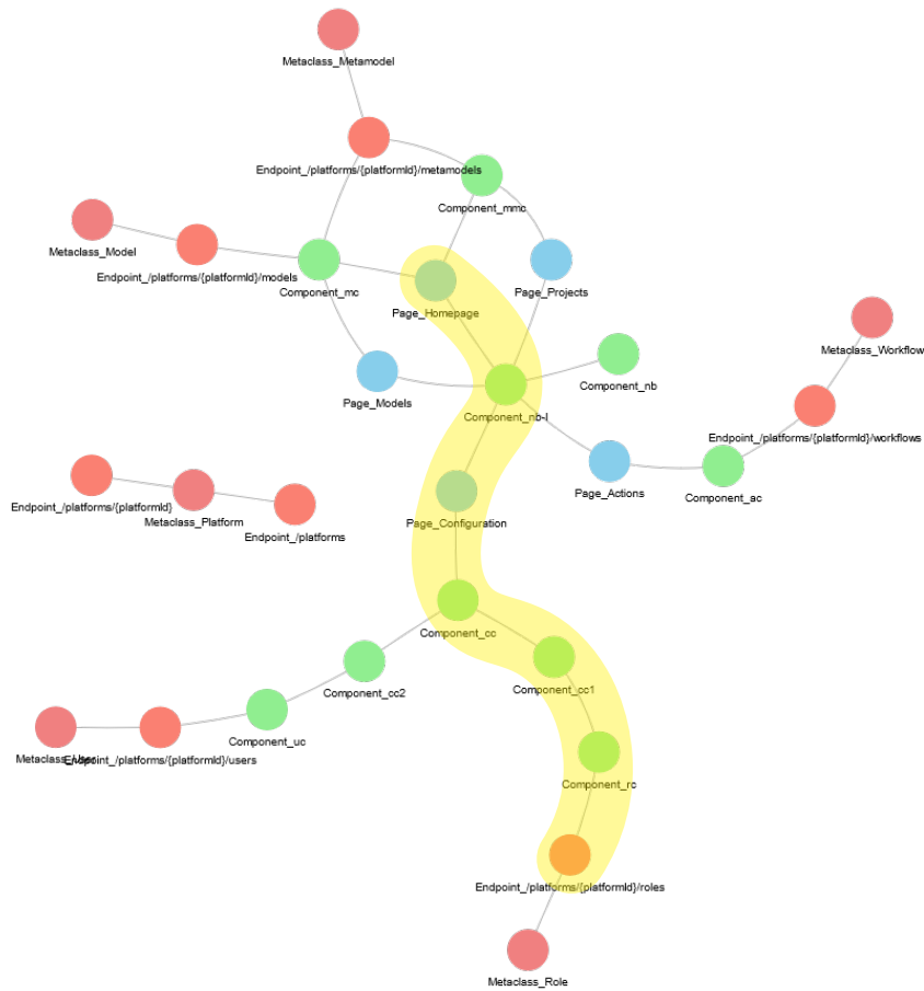
Figure 4: A LowcoBot model flattened to a graph, as consumed by the Navigation tool. Highlighted is the shortest path between the homepage and a Role endpoint. The path is computed to answer the question Where can I change roles? Legend: blue = Webpage, green = (Abstract)Component, salmon = Endpoint, red = LinguisticConcept.
